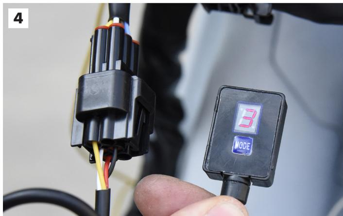
**Map 3** – increase of the engine rpm to 10.000 + Polini 78,8 cylinder kit + Polini upgrade gears + springs valves + if you use the original variator replace the original rollers with the 7gr ones.
