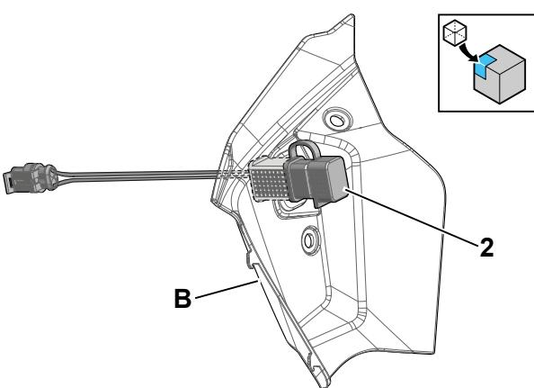
**GB** Fit the USB port 2 on the rubber gasket 1 maintaining the cap opened upward.
