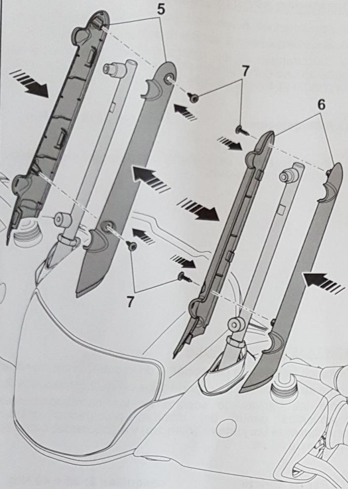
**GB** Fit the covers 5 on the right support rod and the covers 6 on the left support rod, fastening them both with the screws 7 and making sure that the lower edge of the covers is correctly inserted inside the gaskets.
